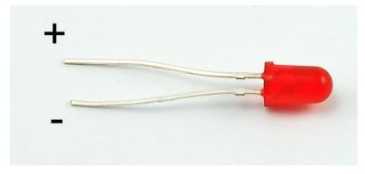
If you do not use a resistor with an LED, then it may well be destroyed almost immediately, as too much current will flow through, heating it and destroying the 'junction' where the light is produced.
