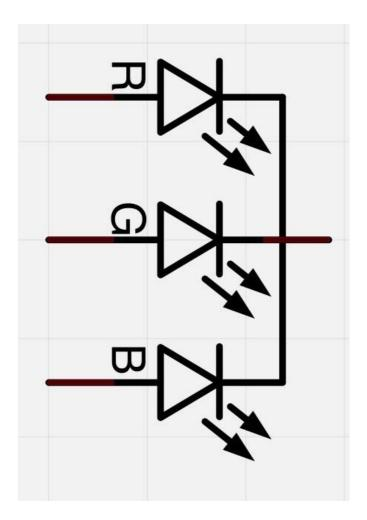
Here on the photographs you can see 4 electrode LED. Every separate pin for Green or Blue or Red color is called Anode. You will always connect "+" to it. Cathode goes to "-"(ground). If you connect it other way round the LED will not light.
