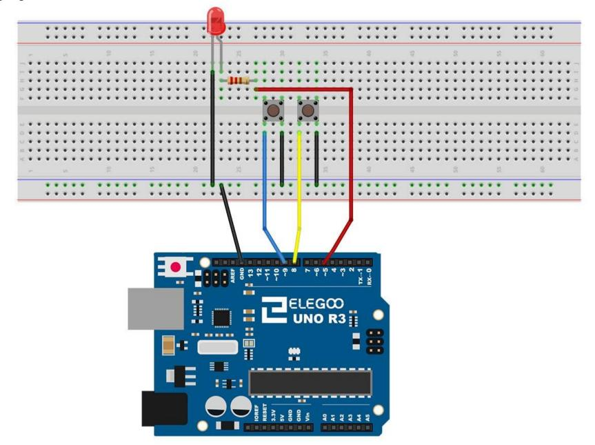
Although the bodies of the switches are square, the pins protrude from opposite sides of the switch. This means that the pins will only be far enough apart when they are placed correctly on the breadboard.
