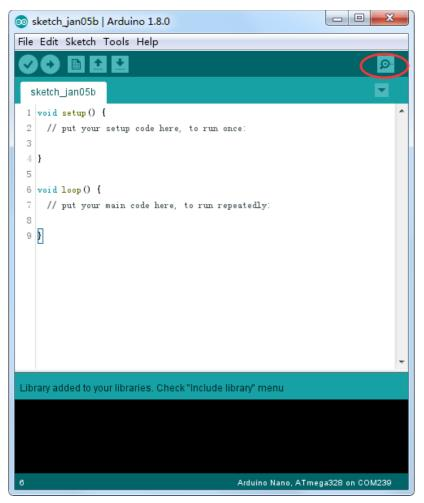
Selecting which port to open in the Serial Monitor is the same as selecting a port for uploading Arduino code. Go to Tools -> Serial Port, and select the correct port. Tips: Choose the same COM port that you have in Device Manager.
