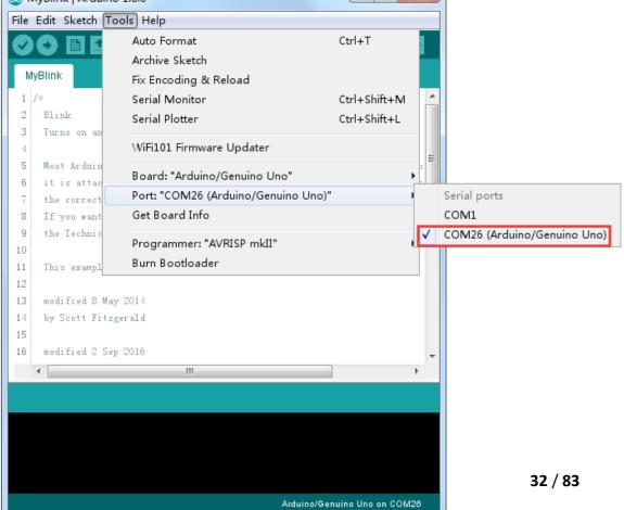
Note: The Board Type and Serial Port here are not necessarily the same as shown in picture. If you are using 2560, then you will have to choose Mega 2560 as the Board Type, other choices can be made in the same manner. And the Serial Port displayed for everyone is different, despite COM 26 chosen here, it could be COM3 or COM4 on your computer. A right COM port is supposed to be COMX (arduino XXX), which is by the certification criteria.
