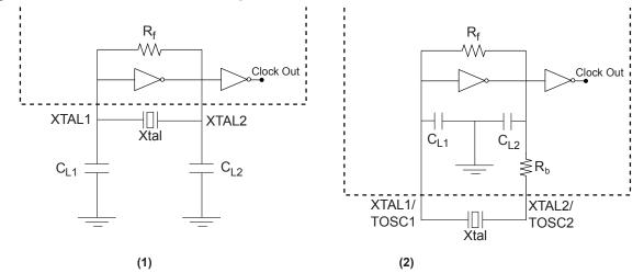
Figure 5-1. Basic Inverter Circuits Equivalent to the Oscillator Circuits in AVR Devices
