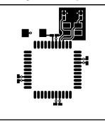
Figure 7-3. ATxmega32A4 - Top Silk Prints of Required/Recommended Connections
