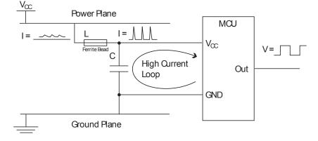
In AVR devices, where power and ground lines are placed close together, there will be better decoupling than in devices with industry standard pinout. In industry standard pinout, the power and ground pins are placed in opposite corners of the DIP package. This disadvantage can be overcome by placing decoupling capacitors very close to the die. For devices with multiple pairs of power and ground pins, it is essential that there is a decoupling capacitor for every pair of pins.
