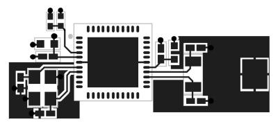
Figure 7-6. ATmega324PB - Top Silk Prints of Required/Recommended Connections
