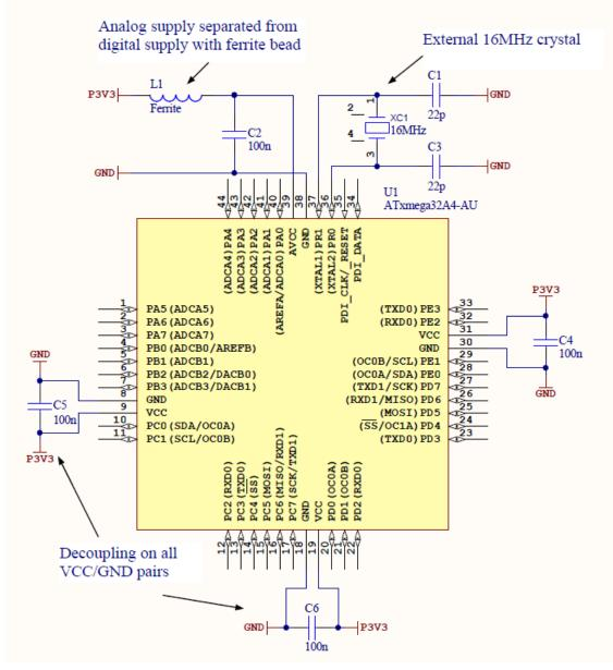
Figure 7-1. ATxmega32A4 - Basic Schematic of Required/Recommended Connections
