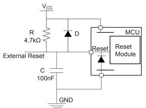
**Note:** The values of resistor R and capacitor C are typical values used for the RESET pin. For specific design requirements of an application, these values must be changed accordingly.
