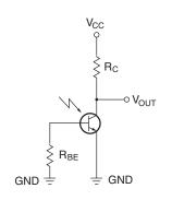
Finally, the phototransistor should be biased (voltage applied to  $V_{CC}$ ) with 5 Volts. The maximum bias is 16 V, however the performance of the component doesn't change with a greater bias except when the phototransistor is used as a switch -- the high level output will equal the higher setting.
