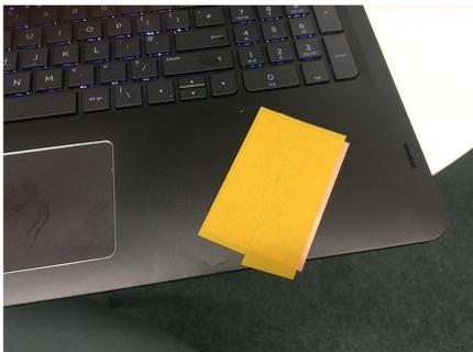
Then stick your board onto the wax spacer (without the wax spacer the mill won't reach the board as it's too high). Overlap the board very slightly with the edge of the wax block to allow us to remove it afterwards.
